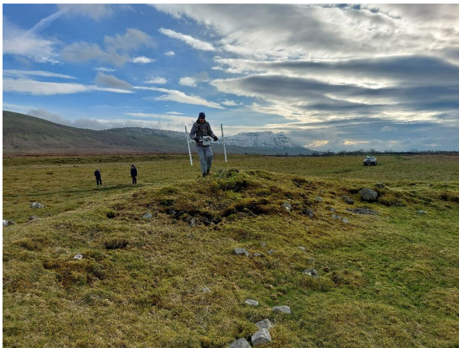
Figure 4 Rick Peterson of UCLAN in full stride with the Bartington fluxgate magnetometer.
