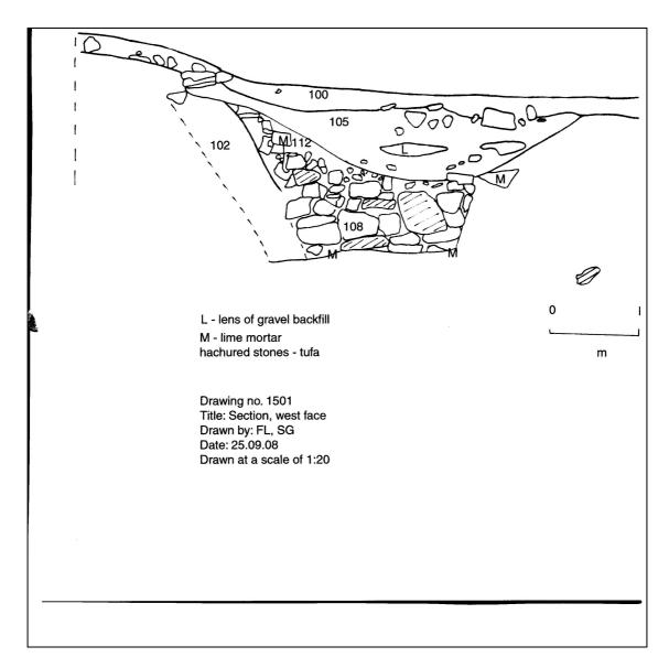
Fig. 10 Section 1501, showing west face of trench
