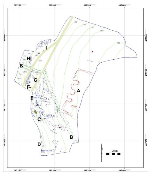
Fig. 4 Topographical survey with features discussed in the text *Red dots indicate the survey reference points. Contours at 2m intervals above OD.*
