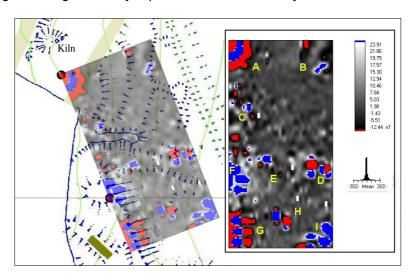
Fig. 7 Processed gradiometer plot of the mill area (despiked and interpolated (SinX/X)) also shown in conjunction with the topographical survey
