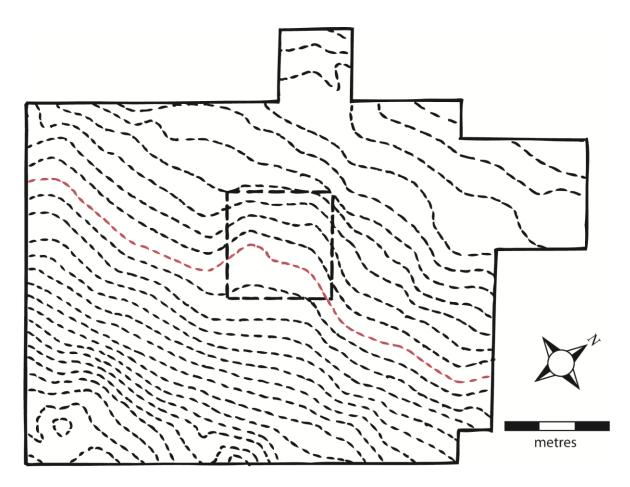
Fig. 11: Contour plot of Trench 8 (contours at 0.1m intervals). Red contour at 320m. Topography dips N-S
